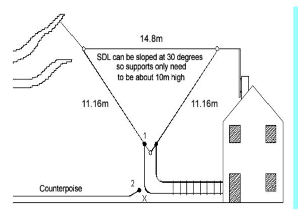
Quarter wave counterpoise can be in a straight line or bent to fit shape of garden. Feeder conductor is connected to point 1 when antenna is fed as a loop (i.e. 3.5-28Mhz) and point 2 when antenna is used on 1.8 Mhz.
