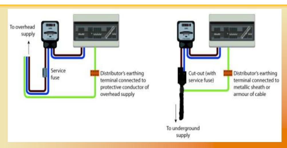
This shows the typical arrangements of the TN-S system for overhead line supply or underground cable supply.
