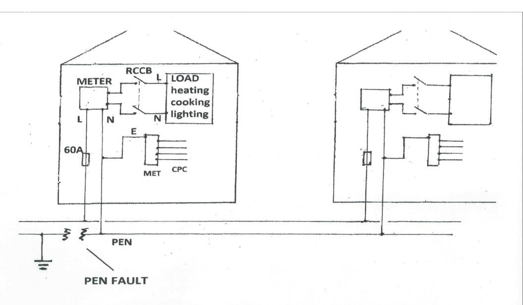
The PEN neutral has been cut but the live is still active. If any of the loads are switched on then the neutral from the loads to the RCCB will be, live so the earth of the MET will also be live. So now everything in the house will be live eg cooker, washing machine, fridge etc. In this case the inside of the house can be considered a Faraday Cage and is accepted as being safe.
