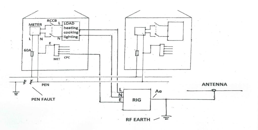
We now have a rig plugged into the ring main so now the chassis of the rig will be at 230V. If the shack is outside the house then Joe is in real danger.
