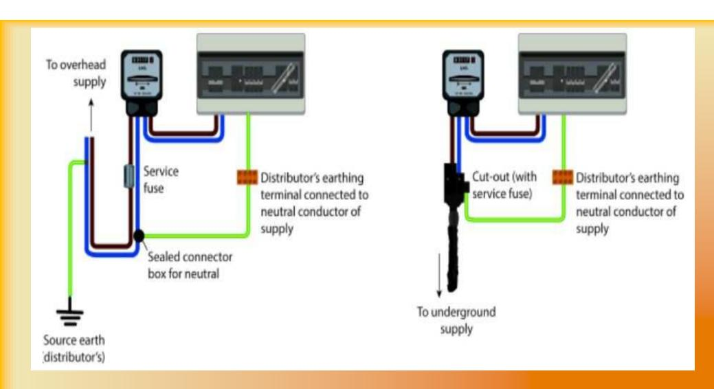
This shows the typical arrangement of the TN-C-S system.
